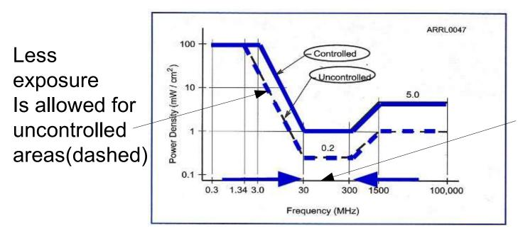
Least exposure is allowed from 30MHZ to 300MHZ where wavelengths are similar to dimensions on humans.
